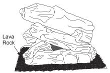
Figure 29 - Installing Lava Rock
